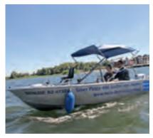
The Silver Pirate 490 is designed to meet the needs of anglers: four rod holders and a built-in small wet storage basin, a comfortable seat, optimal electronics for fishing and plenty of space for fishing equipment. With the flat bottom made of seawaterresistant aluminium, it can run aground on the beach, the robust material can sometimes take a bump without being damaged.
